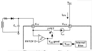
Figure 14. Startup Circuit
