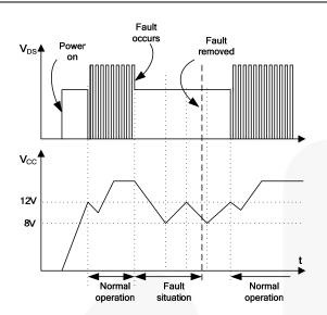
Figure 17. Auto-Restart Protection Waveforms
