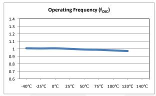
Figure 4. Operating Frequency vs. Temperature
