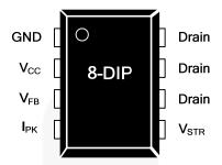
Figure 3. Pin Configuration
