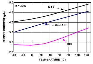
FIGURE 23. ISL28271 SUPPLY CURRENT DISABLED vs TEMPERATURE,  $V_+, V_- = \pm 2.5 V, V_{|N} = 0 V$
