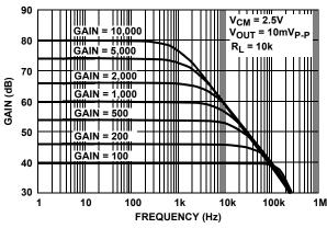
FIGURE 4. ISL28272 FREQUENCY RESPONSE vs CLOSED LOOP GAIN,  $V_{CM} = 1/2V_{+}$
