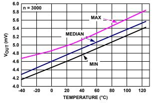
FIGURE 35. ISL28271  $V_{OUT}$  LOW vs TEMPERATURE,  $R_L$  = 100k,  $V_+$ ,  $V_-$  = ±2.5V
