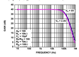
FIGURE 8. ISL28272 FREQUENCY RESPONSE vs SUPPLY VOLTAGE
