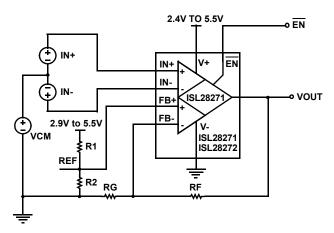
FIGURE 38. GAIN SETTING AND REFERENCE CONNECTION
