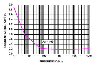
FIGURE 18. ISL28272 INPUT CURRENT NOISE SPECTRAL DENSITY
