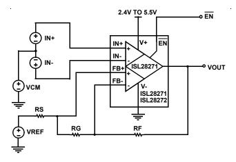
FIGURE 39. REFERENCE CONNECTION WITH AN AVAILABLE VREF
