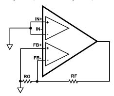
FIGURE 40. PREVENTING OSCILLATIONS IN UNUSED **CHANNELS**
