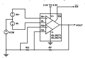
FIGURE 37. GAIN IS SET BY TWO EXTERNAL RESISTORS,  $\rm R_F$  AND  $\rm R_G$
