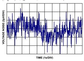
FIGURE 20. ISL28272 0.1Hz TO 10Hz INPUT VOLTAGE NOISE, GAIN = 100
