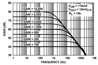
FIGURE 6. ISL28272 FREQUENCY RESPONSE vs CLOSED LOOP GAIN, V<sub>CM</sub> = V<sub>-</sub>
