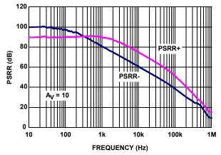
FIGURE 13. ISL28271 PSRR vs FREQUENCY
