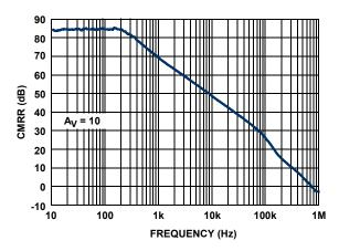
FIGURE 11. ISL28271 CMRR vs FREQUENCY
