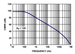
FIGURE 12. ISL28272 CMRR vs FREQUENCY
