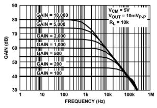
FIGURE 2. ISL28272 FREQUENCY RESPONSE vs CLOSED LOOP GAIN,  $V_{CM} = V_{+}$
