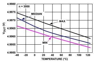
FIGURE 31. ISL28271  $V_{OUT}$  HIGH vs TEMPERATURE,  $R_L$  = 100k,  $V_+$ ,  $V_-$  = ±2.5V
