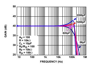
FIGURE 10. ISL28272 FREQUENCY RESPONSE vs C<sub>LOAD</sub>
