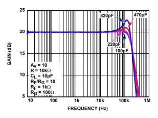
FIGURE 9. ISL28271 FREQUENCY RESPONSE vs C<sub>LOAD</sub>
