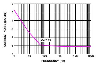
FIGURE 17. ISL28271 INPUT CURRENT NOISE SPECTRAL DENSITY
