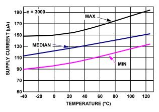
FIGURE 21. ISL28271 SUPPLY CURRENT ENABLED vs TEMPERATURE,  $V_+, V_- = \pm 2.5 V, V_{IN} = 0 V$
