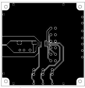
L1 : Copper wiring pattern diagram
