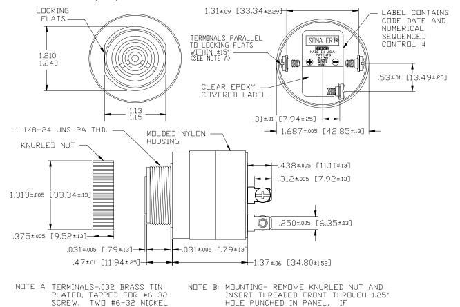
PRODUCES TWO TONES ALTERNATELY WHEN USED WITH ADDITIONAL CONTINUOUS UNIT
