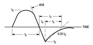
Figure 14. Diode Reverse Recovery Waveform
