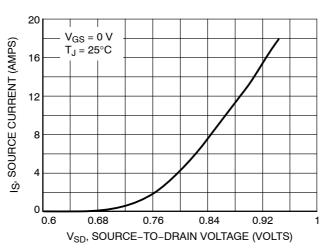
Figure 10. Diode Forward Voltage versus Current
