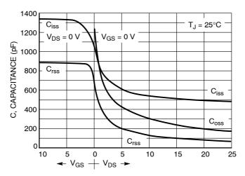
GATE-TO-SOURCE OR DRAIN-TO-SOURCE VOLTAGE (VOLTS)
