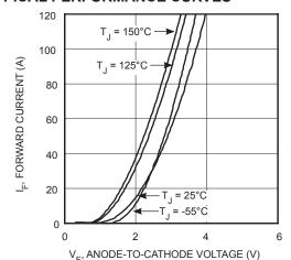
FIGURE 19, F Forward Current vs. Forward Voltage
