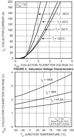
FIGURE 5, On State Voltage vs Junction Temperature
