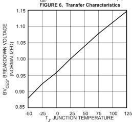
FIGURE 8, Breakdown Voltage vs Junction Temperature
