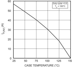
FIGURE 24, Max Average Forward Current vs. CaseTemperature
