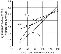
FIGURE 23, Dynamic Parameters vs. Junction Temperature
