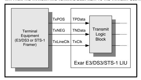
The manner that the LIU handles Dual-Rail data is described below and illustrated in Figure 15. The Transmit Section (of a Channel) typically samples the
