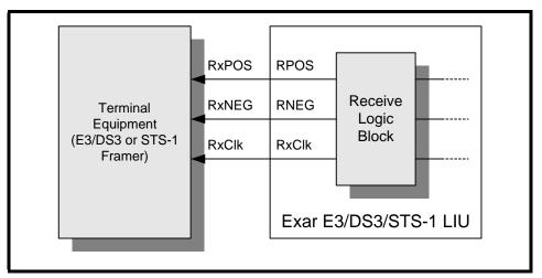
The manner that a given channel transmits Dual-Rail data to the Receiving Terminal Equipment is de-
