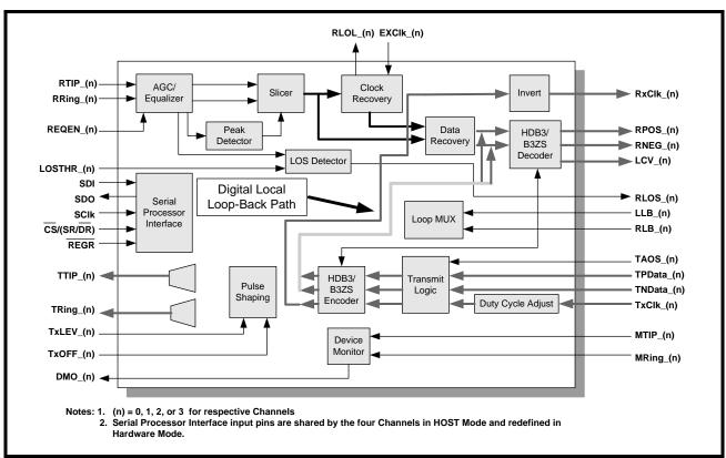
Configure a channel to operate in the Digital Local Loop-Back Mode by employing either one of the following two-steps:
