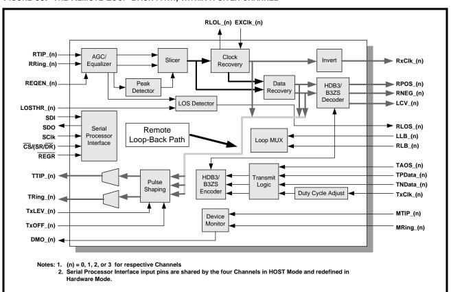
Configure a channel to operate in the Remote Loop-Back Mode by employing either one of the following two steps
