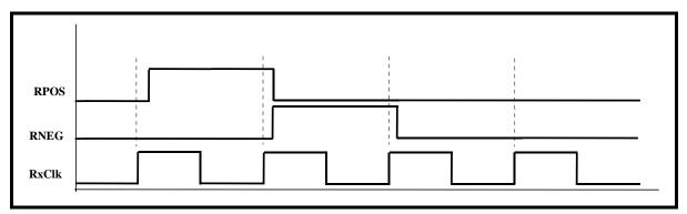
RxClk\_(n) is the Recovered Clock signal from the incoming Received line signal. As a result, these clock signals are typically 34.368 MHz for E3 applications, 44.736 MHz for DS3 applications and 51.84 MHz for SONET STS-1 applications.
