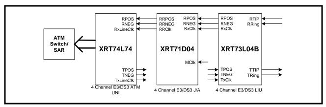
FIGURE 3. MULTISERVICE - FRAME RELAY APPLICATION
