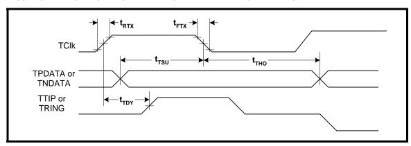
FIGURE 7. TIMING DIAGRAM OF THE RECEIVE TERMINAL OUTPUT INTERFACE
