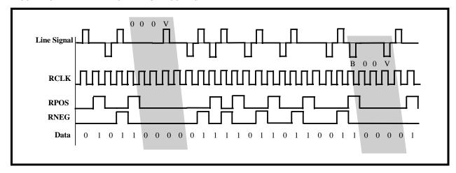
**Note:** If the HDB3 Decoder detects any bipolar violation (e.g., "V") pulses that is not in accordance with the HDB3 Line Code format, or if the HDB3 Decoder detects a string of 4 (or more) "0's" in the incoming line signal, then the HDB3 Decoder flags this event as a Line Code Violation by pulsing the LCV output pin "High".
