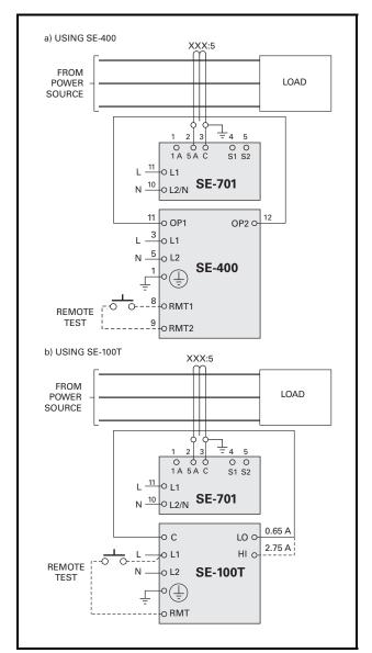
FIGURE 12. Ground-Fault-Test Circuits.
