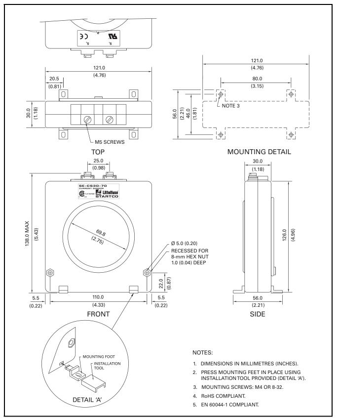
FIGURE 7. SE-CS30-70 Current Sensor.
