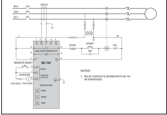
FIGURE 3. Typical Three-Phase-Starter Connection.
