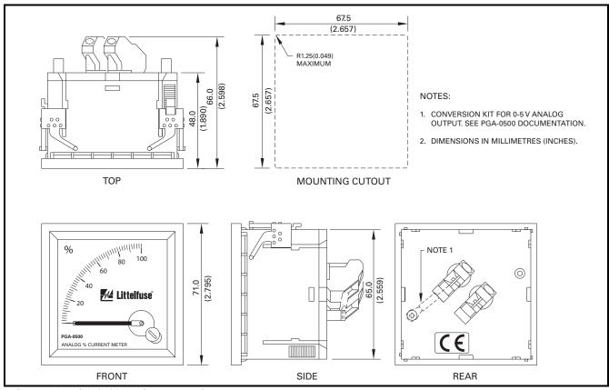
FIGURE 11. PGA-0500 Analog Percent Current Meter.
