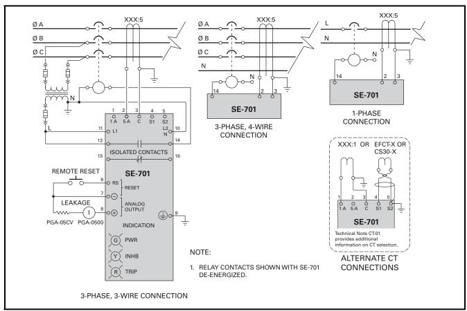
FIGURE 2. Typical Connection Diagrams.
