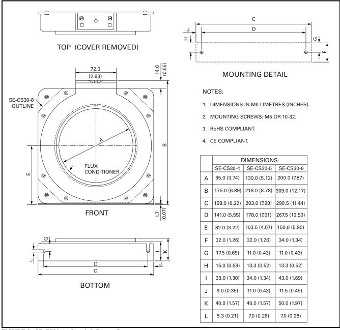
FIGURE 8. SE-CS30-4, -5, and -8 Current Sensors.
