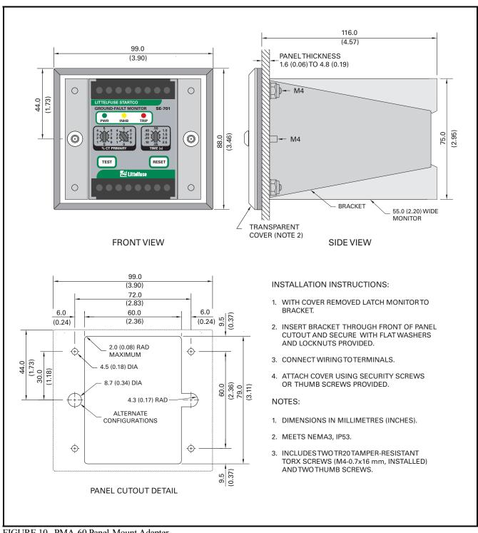
FIGURE 10. PMA-60 Panel-Mount Adapter.
