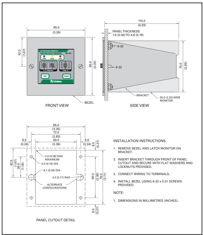
FIGURE 9. PMA-55 Panel-Mount Adapter.
