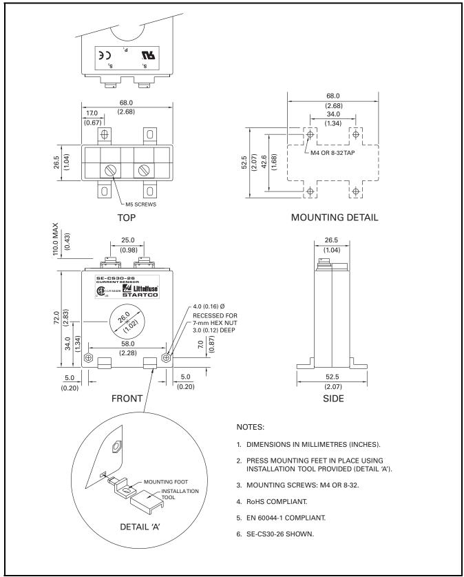
FIGURE 6. EFCT-26 and SE-CS30-26 Outline and Mounting Details.
