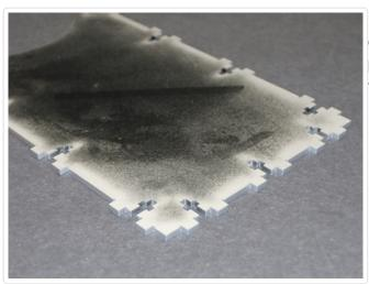
Because T-slot construction was used, the edges of the main spine need special attention. They'll be poking through the frame sides, so the edges of this one piece were also painted to match.
