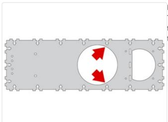
**Be extra careful** with the large main "spine" piece. The plastic is quite thin between the eye hole and two particular T-slots. It's not a problem once all the supporting pieces are added.
