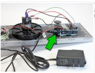
The 9V power source (whether battery or AC adapter) connects to the DC jack on the Arduino board.
