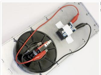
LEDs have a specific *polarity*. You may need to switch battery terminals to get it to light.
