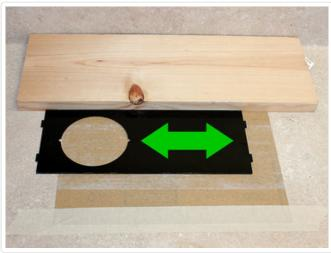
finish. A full sheet of 220 grit sandpaper (\$1.25) is taped face-up to the workbench, while a scrap of wood provides a straight edge to work against.
