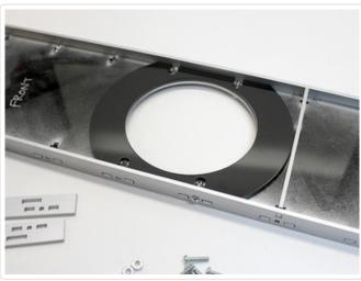
This spacer ring makes the unit feel more solid, so it doesn't cave in when the button is pressed. Note that it's not quite symmetrical — there's a definite "up" and "down" due to the T-slots.
