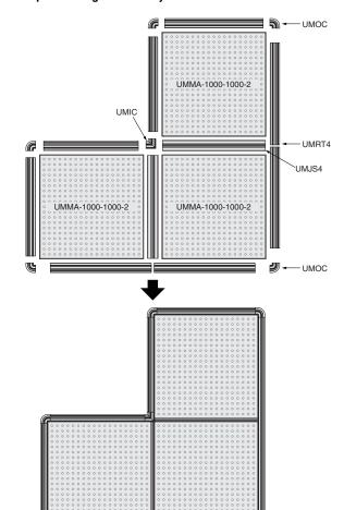
In this case, the perimeter of the Safety Mat is about 8 m, the joint between the Safety Mats is 2-m long, and the following pieces are required:
