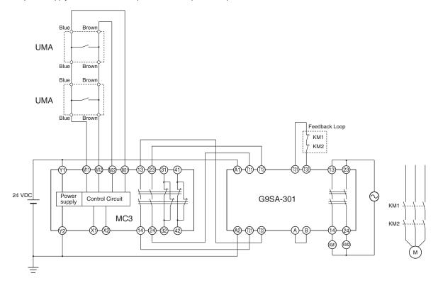
KM1, KM2: Magnetic contactor M: Motor
