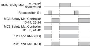
Note: Remove the three yellow jumpers from the MC3 to use Manual Reset Mode. Refer to Mat Controller MC3 Series Installation and Operating Manual for the location of the jumpers.
