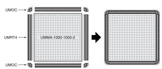
In this case, the perimeter of the Safety Mat is about 4 m and the following pieces are required:
