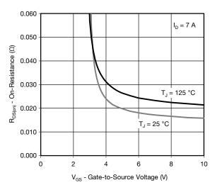
On-Resistance vs. Gate-to-Source Voltage
