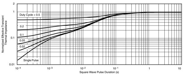
Normalized Thermal Transient Impedance, Junction-to-Foot
