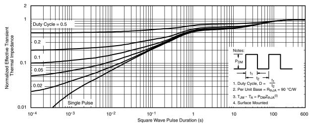
Normalized Thermal Transient Impedance, Junction-to-Ambient
