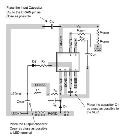
Figure 2. PCB Layout Guide
