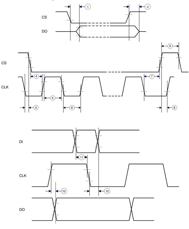
Inputs DI, CLK, CS: High level = 0.7  $\times$  V $_{\rm CC}$ , low level = 0.3  $\times$  V $_{\rm CC}$  Output DO: High level = 0.8  $\times$  V $_{\rm CC}$ , low level = 0.2  $\times$  V $_{\rm CC}$
