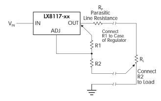
FIGURE 3 — CONNECTIONS FOR BEST LOAD REGULATION
