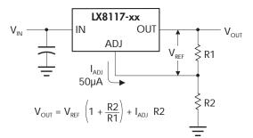
FIGURE 2 — BASIC ADJUSTABLE REGULATOR
