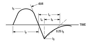
Figure 14. Diode Reverse Recovery Waveform
