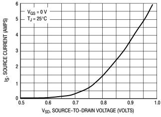
Figure 10. Diode Forward Voltage versus Current
