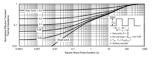
Normalized Thermal Transient Impedance, Junction-to-Ambient
