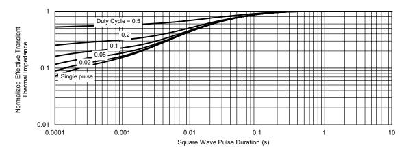
Normalized Thermal Transient Impedance, Junction-to-Case
