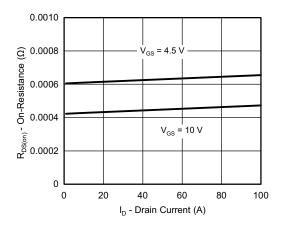
**On-Resistance vs. Drain Current and Gate Voltage**
