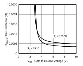
On-Resistance vs. Gate-to-Source Voltage
