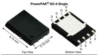
**PRODUCT SUMMARY**  $V_{DS} \overline{(V)}$ 25  $R_{DS(on)}$  max. ( $\Omega$ ) at  $V_{GS}$  = 10 V 0.00058  $R_{DS(on)}$  max. ( $\Omega$ ) at  $V_{GS}$  = 4.5 V 0.00082 Qg typ. (nC) 61 100 <sup>a, g</sup> I<sub>D</sub> (A) Configuration Single
