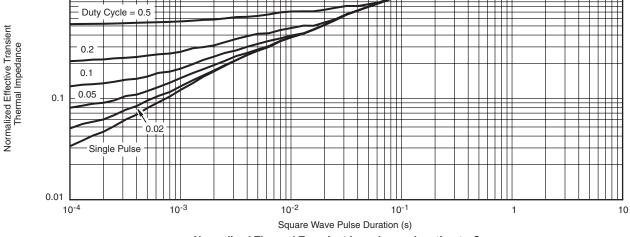
Normalized Thermal Transient Impedance, Junction-to-Case
